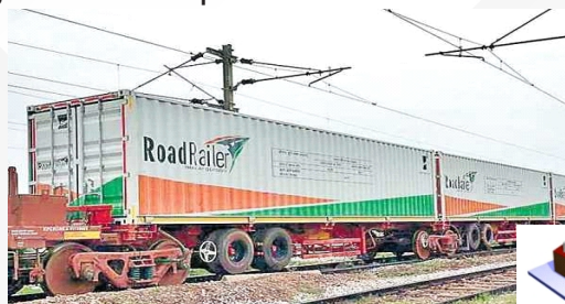
RoadRailer – A wagon with tyres and wheels for rail tracks
